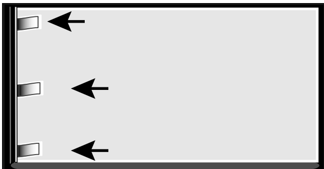
Step 1. Diamond Shield molding clip removal
